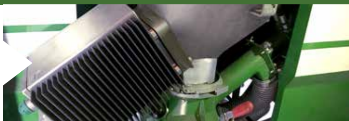
POLYTEC NIR spectrometer system on a HALDRUP F-55 green forage harvester
